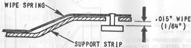
Fig. 11.—Section of flame detector stationary contact. Both the hot and cold side contacts have wipe or follow . The contact itself is mounted on a wiper spring of phosphor bronze and this is held by a heavier support strip. In operation , when the movable contact pushes against this contact it can move it about .015 inch. However, if the wiper spring be stiff, and the clutch slip very easily, the movable contact may not be able to take up the wiper. This is important on the hot side, for then the slightest fluctuation in temperature may break the circuit, and the furnace will recycle. Sometimes tightening the clutch spring (sliding it closer to the clutch) will cure this. Also make sure there is no grease on the clutch. Dirt or corrosion behind the contact may also cause insufficient wipe by limiting the movement. Wipe is also lost if the wiper spring become bent so that the contact stays back against the support strip and therefore has no movement.
